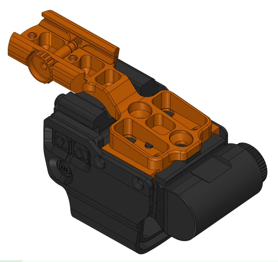
Progressively tighten new base screws while firmly pressing driver bit into T25 socket.
