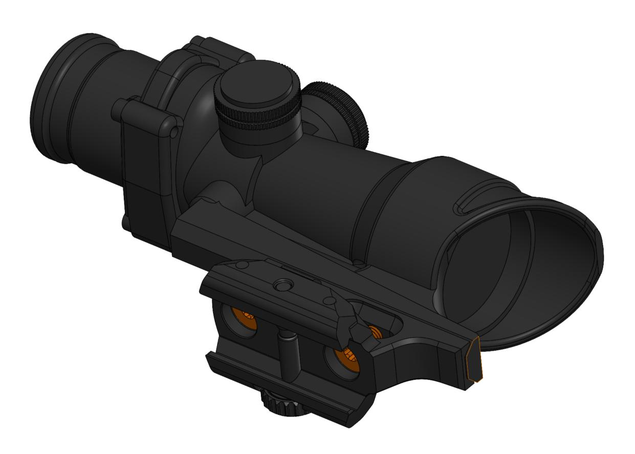
Progressively tighten each screw while firmly pressing driver bit into T25 socket
