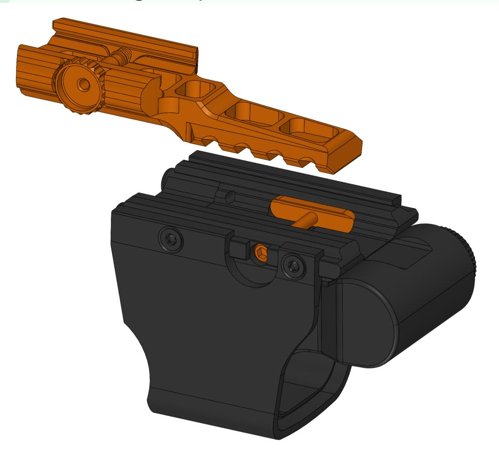
O2. Visually inspect to verify proper seating. Fasten XPS 7/64" hex bolt to 17 inch-lbs.
