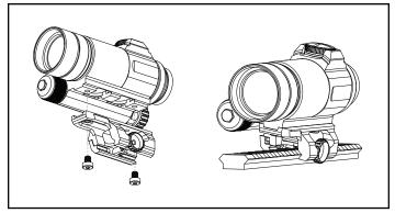
1. Attach optic onto Low Drag Mount by tightening supplied Nylok® Torq-Patch® treated screws, in an alternating pattern, to 37in-lbs, using a 3mm hex socket driver.
